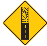
Pavement ends ahead
